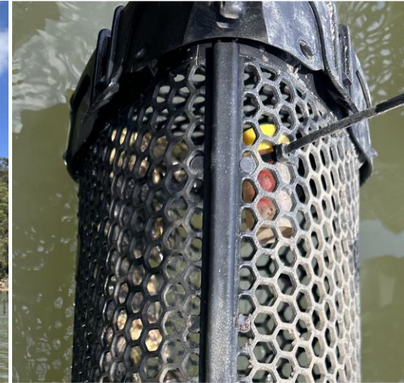
USYD temp probes in baskets
