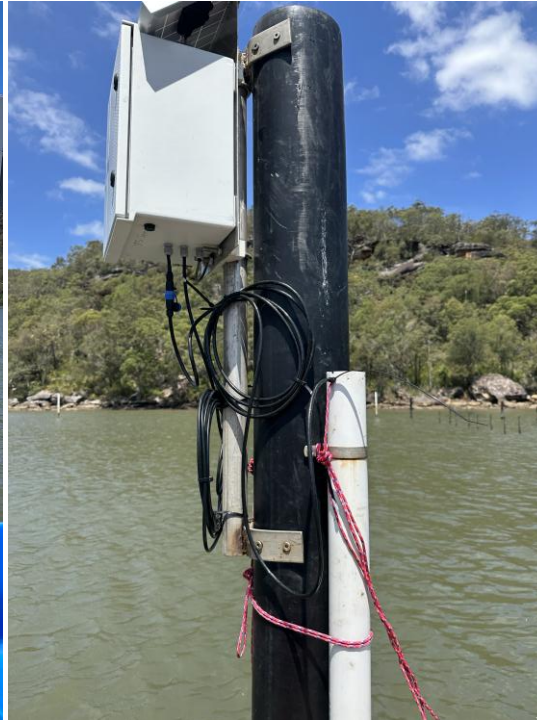
ICT-DPI Probe at Porto + USYD oxygen, salinity and bar pressure probes
